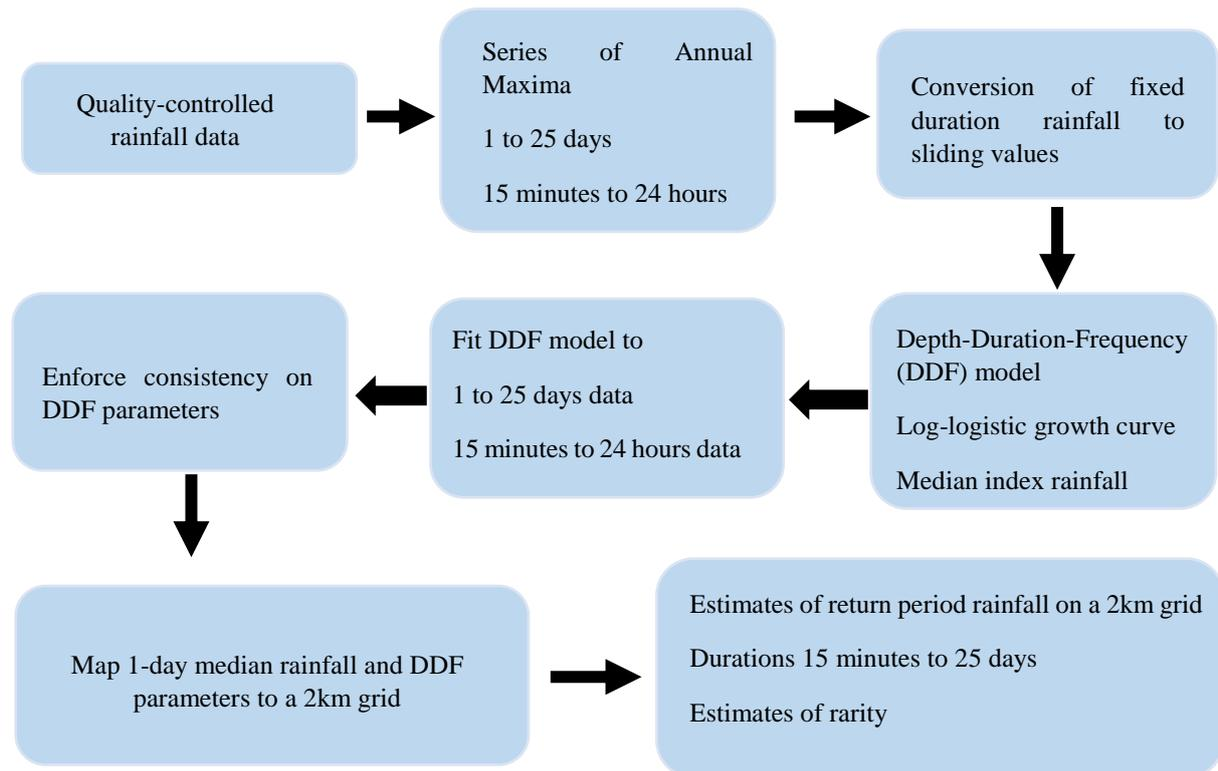
Figure 6: Workflow of the methodology employed in this study.
